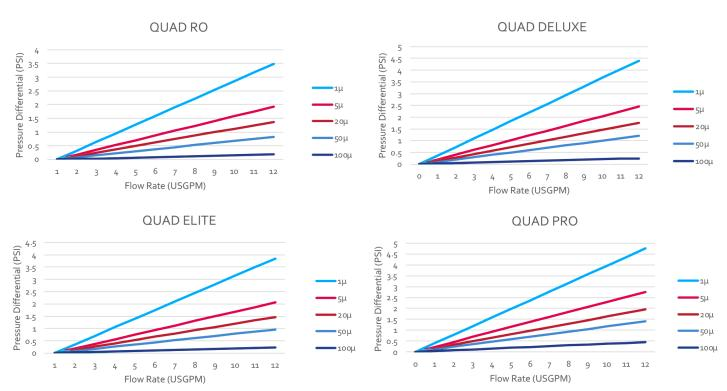
This chart exemplifies normal flow rate for a cartridge length of 10" with water at an ambient temperature as the test fluid. Cartridge length does not cause change in differential pressure, but increasing flow across the housing does.
