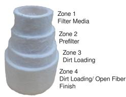
This image shows the Quad Series cut away layer by layer. The outermost layers are made of larger diameter fibers to allow larger particles to flow through, while the inner most layers trap the fine particles maximizing the life of the filter.
